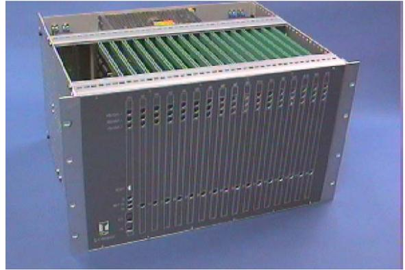
The ET-6416 video matrix switching control unit has 64 video inputs, with full matrix switching to 16 video outputs. Each video matrix switching control unit has RS-422 data communication port. Provides camera title, 24 hour time/date, monitor number and titling displays can be selected by 8 step of grey scale.
